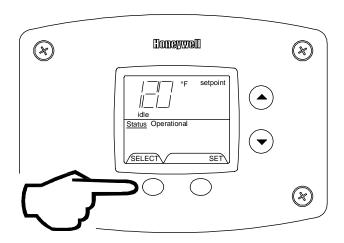
Step 2: Press the "Set" button to enter the setting mode. "Setpoint" will flash in the water heater display.
